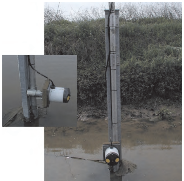
Figure 1-1. H-beam and Speed-Rail™ mount for sidelooker ADVM. (Photographs by Keith Ging, Lower Colorado River Authority; used with permission.)
