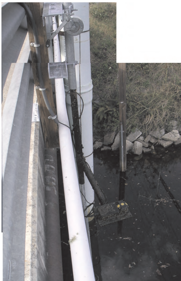
Figure 1-11. ADVM mount with a winch assembly for raising and lowering the ADVM. (Photograph by Jeff Banner, Sarasota County, Florida, Used with permission.)
