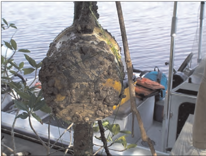
Figure 1-12. Side-looking ADVM with biofouling. (Photograph by Lars Soderqvist, USGS.)
