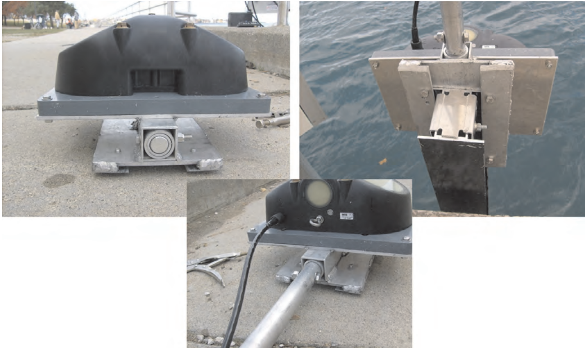
Figure 1-6. ADVM mount for I-beam mounted to channel wall. (Photograph by Don James, USGS.)
