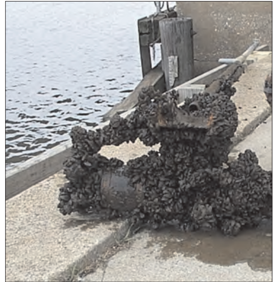
Figure 1-13. Side-looking ADVM coated with zebra mussels. (Photograph by Paul Baker, USGS.)
