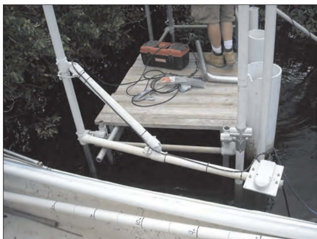
Figure 1-10. Uplooker ADVM mount with ADVM and Speed-Rail™ coated with antifouling paint. (Photograph by Lars Soderqvist, USGS.)
