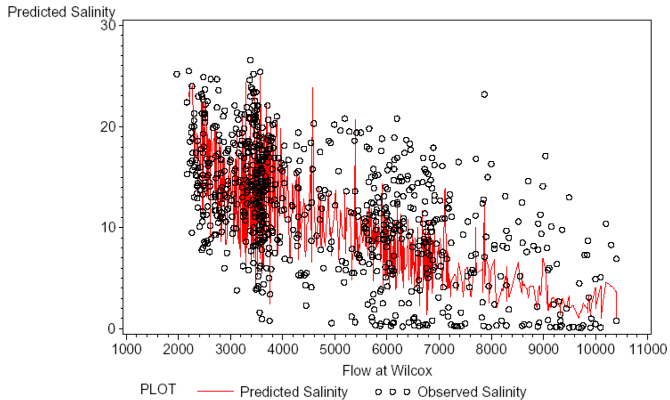
Figure H-7. Predicted and observed daily maximum salinity as a function of flow, based on mid-water column samples.
